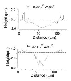
Fig. 3 – Cross-sectional images of the crater for: a – laser irradiance slightly below the phase explosion threshold (20 GW/cm<sup>2</sup>) and b – laser irradiance slightly above the threshold (24 GW/cm<sup>2</sup>) (Schittenhelm *et al.*, 1996).
