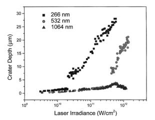
Fig. 2 – Dependence of the crater depth on the incident laser wavelength and irradiance (Schittenhelm *et al.*, 1996).
